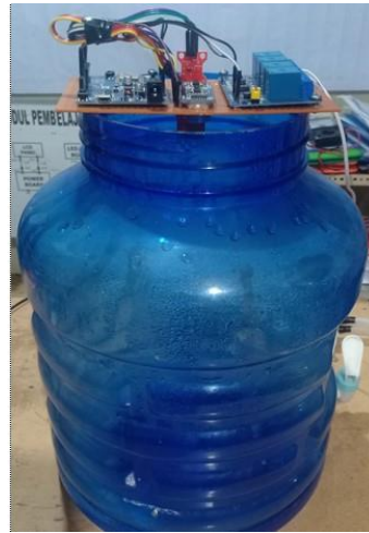
Fig. 7. Installation of a water level control system using an IoT application in a water reservoir
