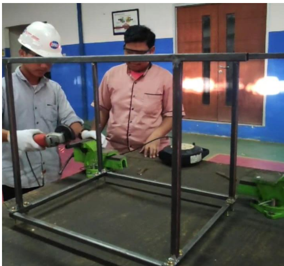
Figure 5. AGV robot frame manufacturing process
