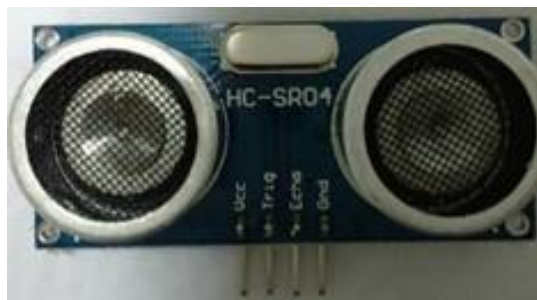
Gambar 5. Sensor PING HC-SR04
